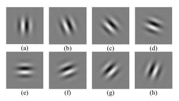
Figure 1. Gabor filters of the same scale and wavelength with different orientations: (a)  $0^{\circ}$ ; (b)  $22.5^{\circ}$ ; (c)  $45^{\circ}$ ; (d)  $67.5^{\circ}$ ; (c)  $90^{\circ}$ ; (c)  $112.5^{\circ}$ ; (c)  $135^{\circ}$ ; (c)  $157.5^{\circ}$ .
